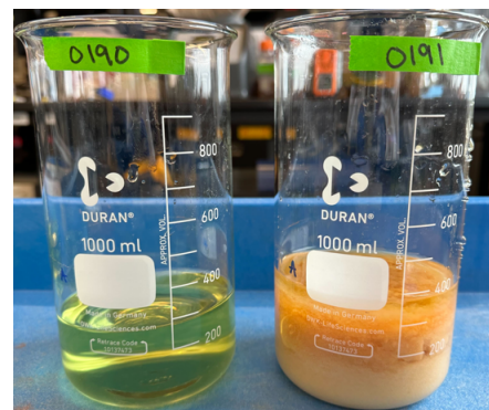
Figure 7. Cations are Readily Precipitated out of the Bio-solvents with Base Adjustment. While
