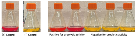
Figure 8. Enzymatic activity observed in select microbes within Allonnia's biobank. Utilization of urea results in a yellow to red color change.
